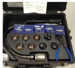
Multihead Hydraulic Swaging Unit- 1/2 to 1 in. and 1 to 2 in. Weekly: $275
